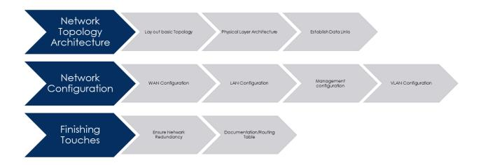
In addition to a Gantt Chart, our group also used an FDD Diagram for project management assistance. The FDD diagram was broken up into three macro areas: Network Topology Architecture, Network Configuration, and Finishing Touches.
